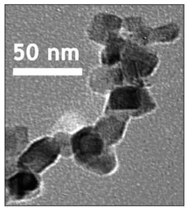
Figure 1. TEM image shows the nanoscale crystalline structure of titanium dioxide in NIST SRM 1898 (color added for clarity.) Credit: Impellitteri/EPA
