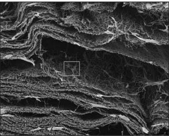
On the cover: SEM visualization of human primary osteoblast colonisation onto a polycaprolactone nanofibrous 3D scaffold after three days. Scale bar:  $150~\mu m$ .
