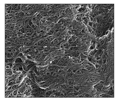
Figure 1. Scanning electron microscope image of a typical sample of the NIST single-wall carbon nanotube soot standard reference material. Recent NIST research suggests that, at least in the laboratory, carbon nanotubes may help protect DNA molecules from damage by oxidation. The image shows an area just over a micrometer wide. (Color added for clarity.)
