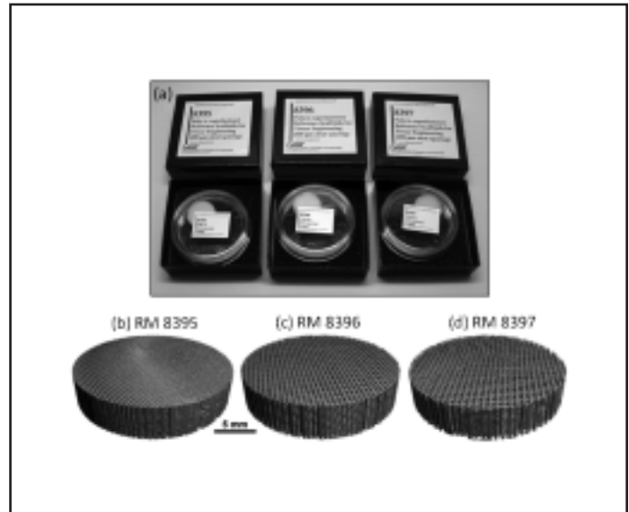
Fig. 1. (a) Picture of NIST Reference Material scaffolds in packaging. (b-d) X-ray microcomputed tomographs of NIST reference scaffolds. All three have a strut diameter of 200 microns, while 8395 has a strut spacing of 200 microns (b), 8396 has a strut spacing of 300 microns and 8397 has a strut spacing of 450 microns.
