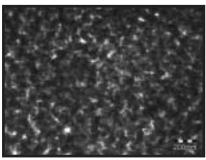
Cover image 2: TEM image of a new dendritic SIBS-type biomaterial with 30 wt% polystyrene content.
