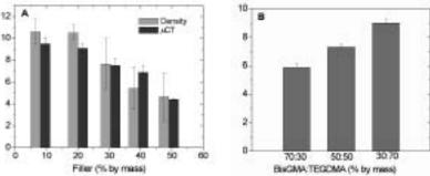
**Figure 1** *A*) Polymerization shrinkage of composites with different filler contents. B) Polymerization shrinkage determined by  $\mu$ CT of composites with constant 30 percent filler and different TEGDMA to BisGMA ratios. Error bars represent one standard deviation (n = 5) and are the estimates of standard uncertainty.
