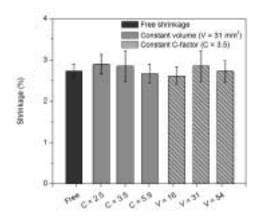
**Figure 2** Polymerization shrinkage determined for unconstrained sample geometries (free) and constrained sample geometries, varying either the *C*-factor or total sample volume. Error bars represent one standard deviation (n = 3) and are the estimates of standard uncertainty.
