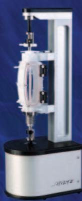
Pulsatile BioDynamic<sup>18</sup> Test Instrument for Vasculat Grafts
