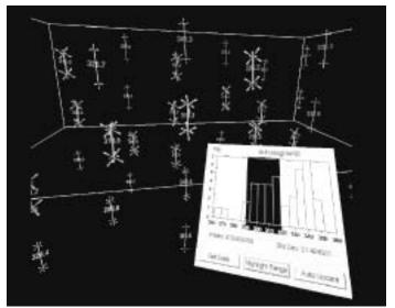
**Figure 4.** Selected histogram bins are highlighted in visualization showing distribution of strut diameters in the range of 200 to 320 lm. The struts have been removed from the scene in order to make the measurements more visible.
