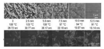
Figure 5. Shown above are a series of six 5 mm \_ 5 mm AFM phase images from a discrete 30/70 DTE/DTO blend film annealed on a variable temperature hot stage for 16 h and the corresponding immuno-fluorescently labeled cells. The spatial arrangement on the surface of the film with the corresponding annealing temperatures and the measured root-mean-square (RMS) roughness data are shown.
