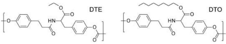
Figure 1. Synthetic scheme and chemical structure of desaminotyrosyl-tyrosine alkyl esters and the resulting polycarbonates. The pendent R groups of the polycarbonates reported in this article consist of ethyl and octyl esters, respectively. The corresponding polymers are referred to as poly(DTE carbonate) and poly(DTO carbonate).
