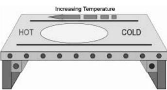
Figure 4. The gradient hot-stage shown above consists of an aluminum (AI) sample plate. Two adjustable AI blocks, with machined heating/cooling channels, are attached to the bottom of the plate. The block channels hold cylindrical heating cartridges or accommodate plumbing for fluid-mediated cooling. The range and slope of the temperature gradient are tailored through the respective block temperatures and their distance apart.
