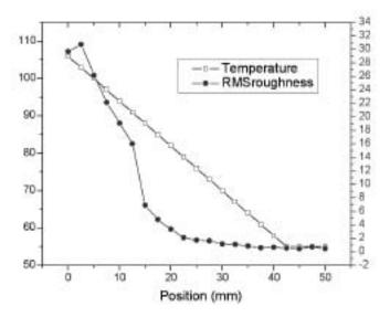
Figure 6. A plot of temperature and RMS roughness vs. position shows both the linearity of the temperature gradient and the distinct drop in RMS roughness that occurs near 90 °C which happens to be the glass transition temperature of DTE (91 °C).
