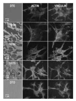
Figure 2. From top to bottom are five 5 mm \_ 5 mm AFM images in which the amount of DTO is increasing. The discrete DTE/DTO blends form phase-separated domains under the prescribed annealing conditions. Immuno-fluorescent staining for actin and vinculin of MC3T3-E1 osteoblasts showing the cytoskeleton and focal adhesion contact formation 16 h after seeding on each of the respective homopolymers and blends. improvement in properties that are preferred over those of the individual components.
