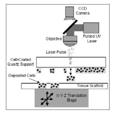
Figure 1. A schematic diagram of a MAPLE DW set up.
