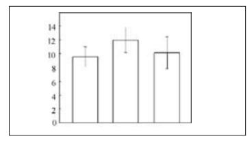
**Figure 1.** Strength of CPC-suture fiber composite made by three different operators to examine operator sensitivity. The three operators produced cements with similar strengths, indicating that the composite fabrication method was reproducible. Horizontal line indicates values not significantly different (p>0.05).
