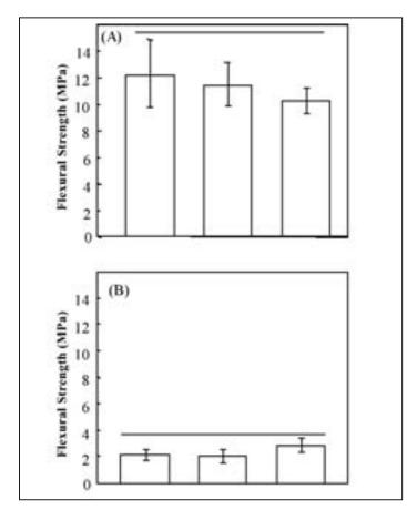
**Figure 2.** Flexural strength of (A) CPC-mesh, and (B) CPC control without mesh, made by three different operators to examine the operator sensitivity. Mesh reinforcement may have potential for craniofacial and thin bone repairs. Horizontal line indicates values that are not significantly different from each other (p > 0.05).
