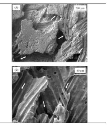
**Figure 2.** SEM of pore channels in CPC-suture fiber composite scaffold after suture fiber dissolution. Arrows indicate the flow of the interconnected pore channels beneath the CPC surface.
