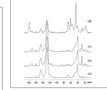
**Figure 1.** The solid state 13C NMR spectra of Fmoc-glycine Wang resin (a), GR(Pbf)GD(Obut)S(But) Wang resin (b), GR(Pbf)GD(Obut)S(But)-initiator Wang resin (c), R(Pbf)GD(Obut)S(But)-poly(HEMA) Wang resin (d).
