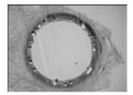
**Figure 5c:** Same poly(DTE carbonate) coated metal stent as in Figure 5b, except that the poly(DTE carbonate) coating delivered an anti-proliferative drug. The drug-eluting formulation reduced neo-intimal hyperplasia.
