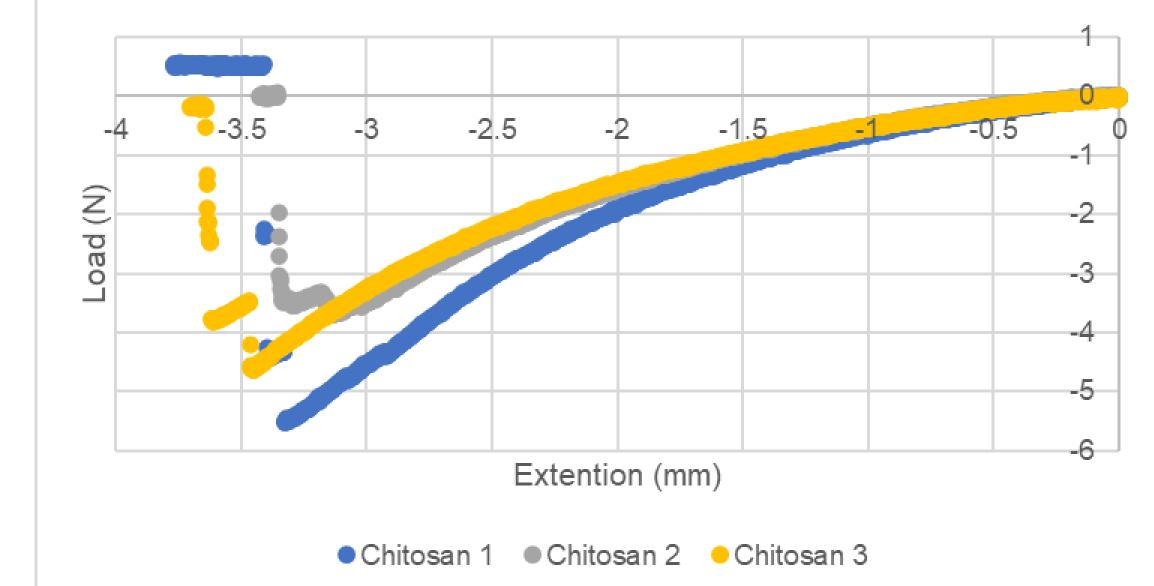
Figure 3. N-MAC-PEGDMA bio-ink replicated test. Rate of compression at mm per min
