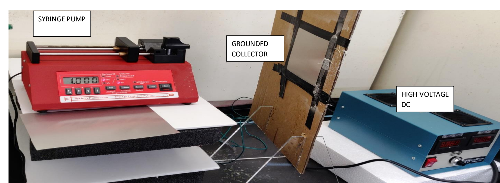
Figure 1. In-house developed electrospinning apparatus with syringe pump(s), grounded collector and a high voltage DC
