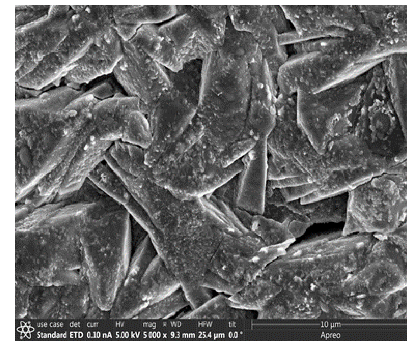
Figure 1. HA crystal formation over NC polymer chains to form a composite material system.
