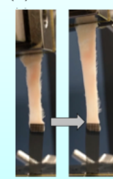
Figure 1. (A) Typical SEM photographs of Ti mesh (pore size, 100 \mu\text{m} ; pitch, 200 \mu\text{m} ) before and after acid treatment. (B) Moisture permeability of the samples after acid treatments. (C) Digital photographs taken during a shear adhesion test of the Ti mesh with a mouse dermal tissue. (D) Shear adhesion strengths of dense and perforated Ti films with different pore sizes. Error bars represent standard deviations ( n=5 ) and the asterisk indicate statistically significant differences with dense Ti film, as determined by a Dunnett test ( p<0.05 ).
